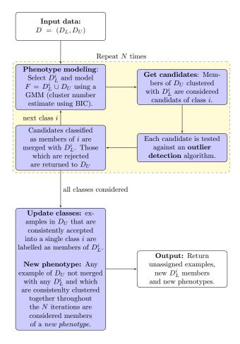
Figure 5: The PhenoDisco iterative algorithm
