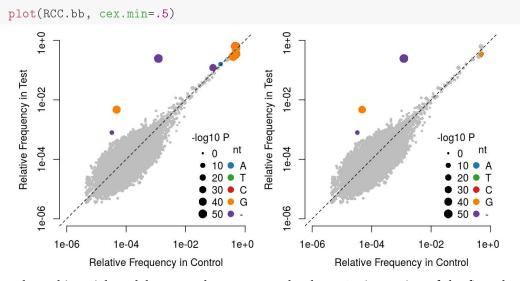
We see that a binomial model was used to generate the data. An inspection of the first plot shows a long noise tail where apparently the dispersion is underestimated causing some false positives. In the second plot we used a beta-binomial model instead and conservatively estimate the dispersion factor on both sides with the argument alternative="two.sided".
