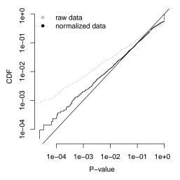
After normalization the cumulative distribution of the p-values is close to the diagonal, even for the smallest values. Hence the p-values accurately measure the probability of type-1 errors.
