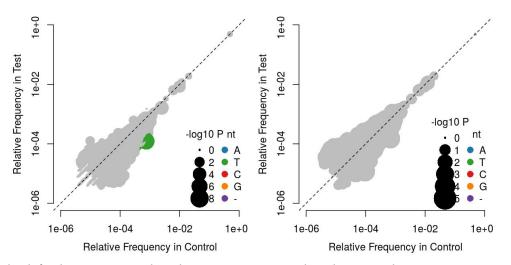
From the left plot it appears that there is a systematic bias between the two experiments, likely because they were sequenced in different runs. The normalized data is shown in the second plot. Now the points now symmetrically scatter around the diagonal and all p-values are within the expected range:
