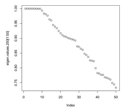
This is "a right" value for normal.sigma because the curve has now a knee shape. Even some variation to this parameter does not change the shape significantly (200 or 300 can be tried).
