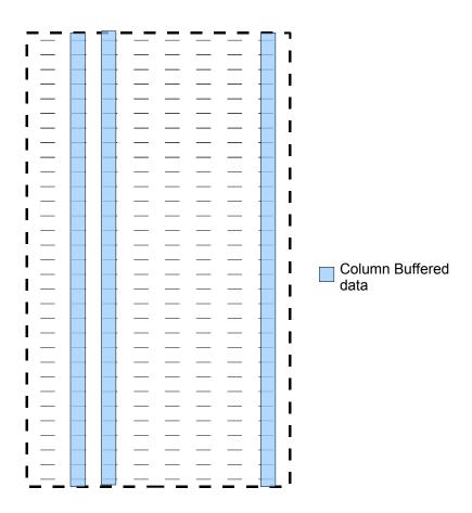
Figure 2: Column Buffers hold selected columns in RAM. This speeds up access to data. Column Buffers are always active
