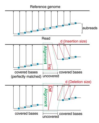
The seed-and-vote paradigm is very powerful in detecting short indels (insertions and deletions). The figure below shows how we use the *subreads* to confidently detect short indels. When there is an indel existing in a read, mapping locations of subreads extracted after the indel will be shifted to the left (insertion) or to the right (deletion), relative to the mapping
