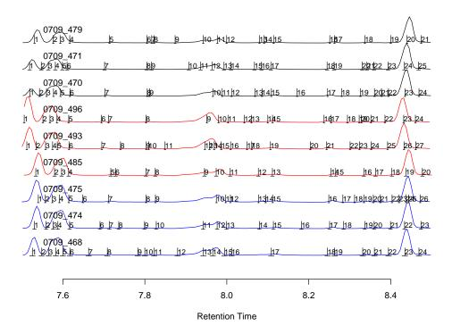
Note here the little *hashes* represent the detected peaks and are labelled with an integer index. One of the main challenges is to match these peak detections across several samples, given that the appear at slightly different times in different runs.
